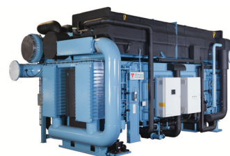
3G Series Capacity: from 176 to 5.300 kW Heat source: Superheated water Superheated water temperature: 180-240°C COP: 1,6-1,9
