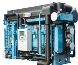
2B series Capacity: from 176 to 12.300 kW Heat source: Steam Steam pressure: 4-10 bar g COP: 1,4
